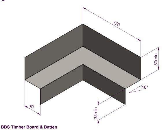
Internal corner 150x150 Flashing @16° for direct fixed
