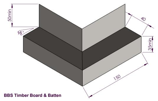
External corner 150x150 Flashing @16° for direct fixed
