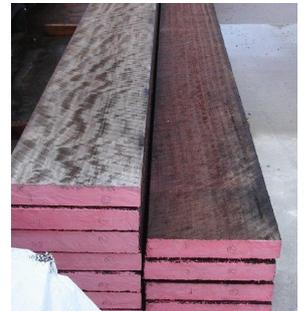
**Mechanical properties:-** High strength in bending, stiffness and crushing categories and medium resistance to shock loads, with a moderate steam bending classification. Bending (fb) 62.77. Compression parallel (fc) 51.21. Tension parallel (tt) 48.25 Shear in beams (fs) 6.2. Compression perpendicular (fp) 15.5. Modulus of Elasticity E(Gpa) 16.55.
