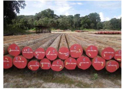
**Mechanical properties:-** Has exceptionally high strength properties even when its weight is taken into account. Weight about 1030kg/m<sup>3</sup> (64lb/ft<sup>3</sup>) seasoned. Bending strength 181 N/mm<sup>2</sup> (26200 lbg/in<sup>2</sup>). Compression parallel to grain 89.9 N/mm<sup>2</sup> (3040 lbg/in<sup>2</sup>)
